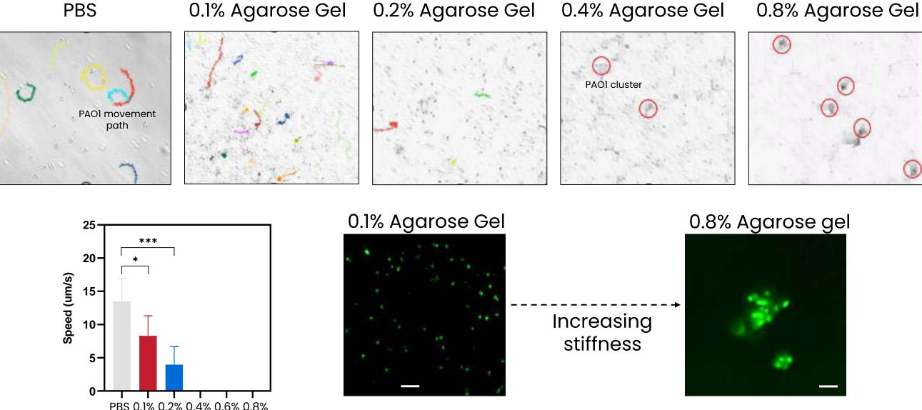
PAO1 cells swim freely in PBS solution but adopt curved paths and become transiently trapped when they are in a gel matrix. Moreover, as gel stiffness increases, the swimming path lengths decrease to the point where cells are locally confined and restricted to rotational movements.
