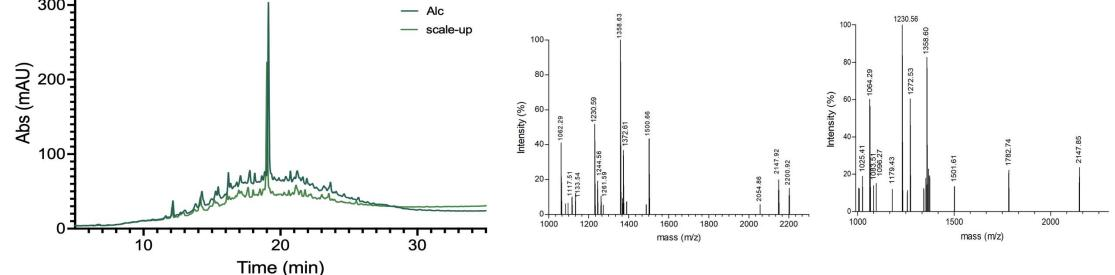
Proteases have been used directly on the raw meal to obtain peptides, which were strategically designed as additives in protein-rich materials. A preliminary screening of the hydrolysates was conducted via RP-HPLC and MALDI-TOF-MS, revealing the formation of hydrophilic peptides with masses ranging between 1000 and 1500 Da. Scale-up of the process was set-up in semi-industrial scale.
