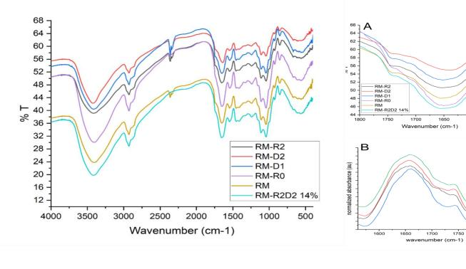
A change in protein structure was evidenced by the FT-IR analysis when comparing the amide I bands of the specimens with different composition to each other and to the one of rapeseed meal, indicating effective protein denaturation. The presence of the reduced disulfide bond and of the denaturing agents causes partial unfolding of the proteins and led to a major exposure of the amino acid side chains in the protein.
