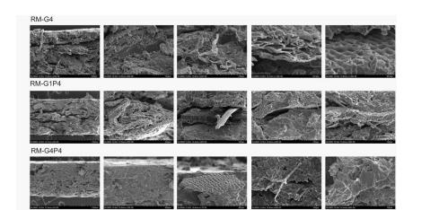
All specimens retain a layered structure, likely due to insufficient applied pressure. However, the G4P4 material exhibits a uniform morphology at 50 and 100  $\mu$ m. Particles of the raw material are still visible to varying degrees.
