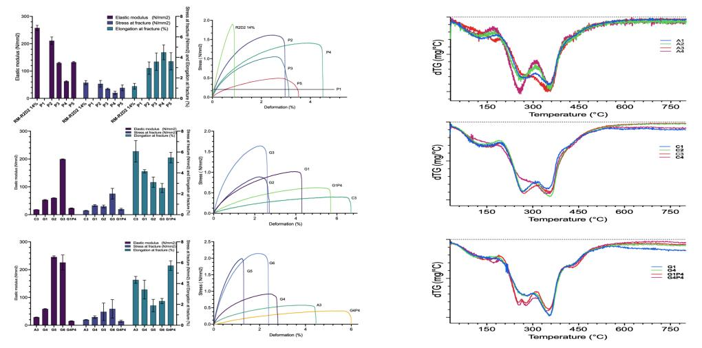
Rapeseed hydrolysates and collagen hydrolysates functioned efficiently as plasticizers due to their hydrophilicity and low molecular weight. Stress-strain analysis indicates a reduction in Young's modulus and a significant increase in elongation at break. Thermogravimetric analysis (TGA) revealed enhanced thermal stability, particularly in materials with a reduced glycerol content in the mixtures.
