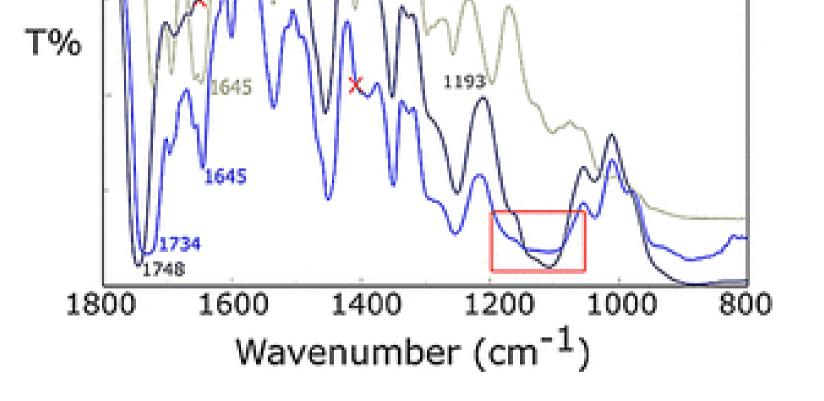
FT-IR analysis. Increase band at 2920–2880 cm<sup>-1</sup> (green region C– H stretching); modification of 1410 cm<sup>-1</sup> band (deformation) C=CH<sub>2</sub>) and the decrease in the intensity of acylic C=O signal (1193 cm<sup>-1</sup>). Broad band (1190– 1050 cm<sup>-1</sup>) of primary alcohols post-reaction.
