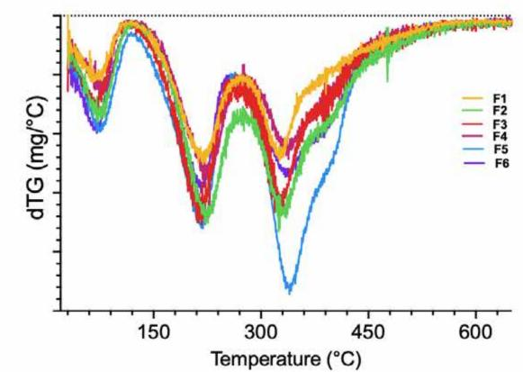
Change in shape in the range of 1600-1625 cm<sup>-1</sup> were observed in the IR spectrum due to changes in the secondary structure of the protein. TGA indicates an enhanced thermal stability for the material containing both the reducing and the denaturing agent (*F6*).
